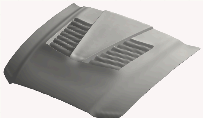
CAD Hood A rebuilt as a mold plug: symmetric, drafted, every feature driven by a parameter.
